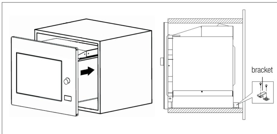
2. Open the door, fix the oven to the cabinet with Screw B through the installation hole. Then fix the trim-kit plastic cover to the installation hole.
